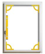
The welded sash frame is tensioned from corner to corner.
