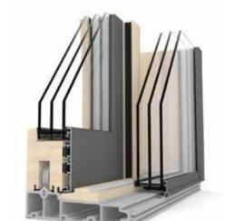
54 mm glazing thickness for standard triple glazing provides best thermal insulation  $U_w$  up to 0.67 W/m<sup>2</sup>K
