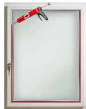
The remaining gap between glass and frame is filled with glue all around.
