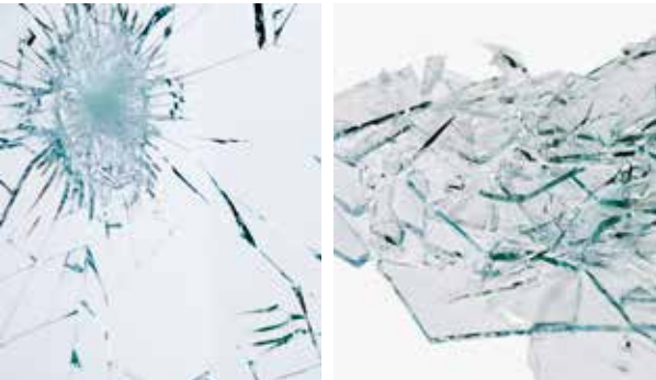
The laminated security glass does not break apart despite using force. Conventional window glass splinters and entry through the window is possible.
